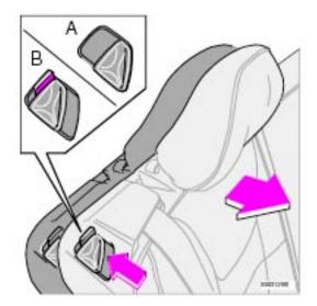
*A* - Catch in closed position.*B* - Catch in open position.
